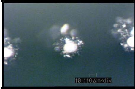
Probe tips before cleaning. (Image from Accretech/TSK UF-200)
