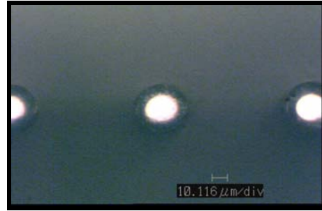
Probe tips after 5 Probe Clean™ insertions. (Image from Accretech/TSK UF-200)
