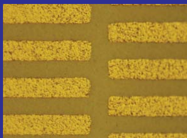
4 micron lines - gold on flex
